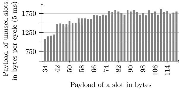
Figure 9: Comparison of the payload per slot and the optimal cumulative payload of unused slots determined by the ILP approach.
